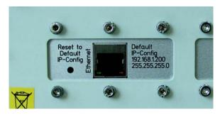
For normal operation the 8140 TETRA AirAnalyzer has to communicate with the controlling application on a PC. This is done using the TCP/IP protocol over the Ethernet.
