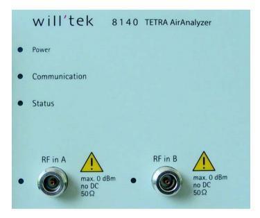
The TETRA AirAnalyzer has two connectors for radio frequency input. Normally you should use RF In A for the downlink (base station transmit) or DMO signal and RF In B for the uplink (mobile station transmit) signal. Both inputs are terminated with 50  $\Omega$  and are limited to a maximum input power of 0 dBm. Proper operation is warranted only without DC voltage.
